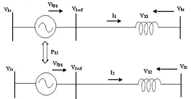
Figure 2. Two-Inverter Interline Power Flow Controller
