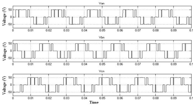
Figure 8. Phase to phase voltages
