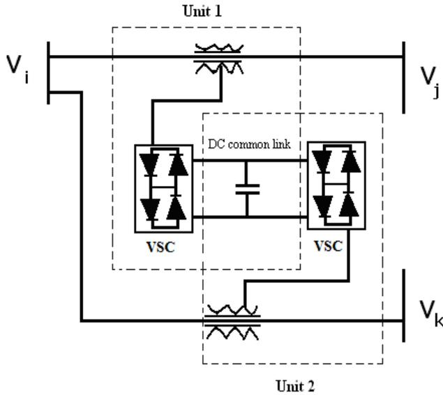
Figure 1. Basic Configuration Of Interline Power Flow Controller
