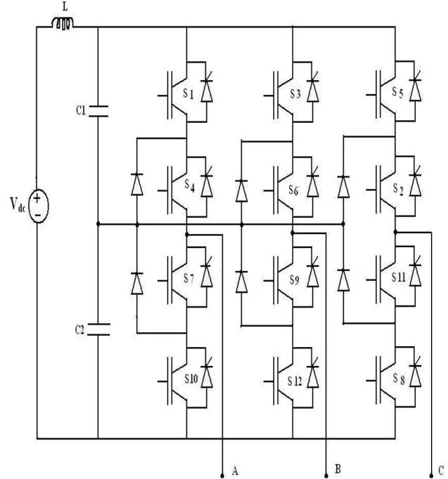
Figure 4. Three level diode clamped inverter
