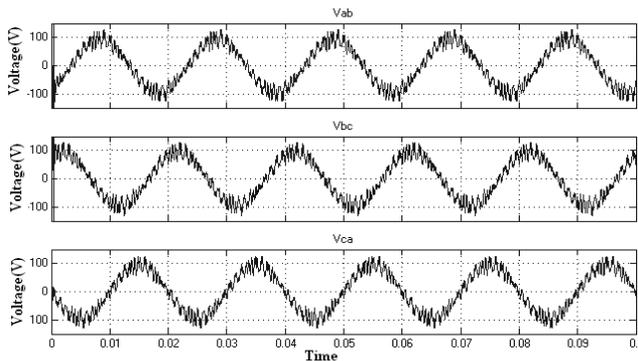
Figure 11. Phase to phase voltages
