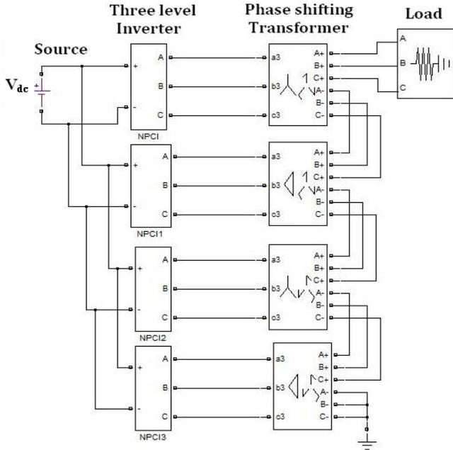
Figure 5. 48-Pulse inverter topology
