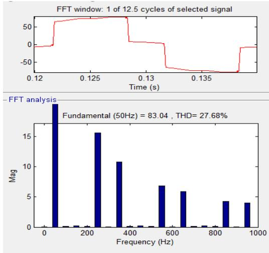
Fig 10.FFT of source current without SVC LIGHT
