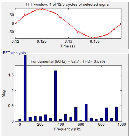
Fig 11.FFT of source current with SVC LIGHT
