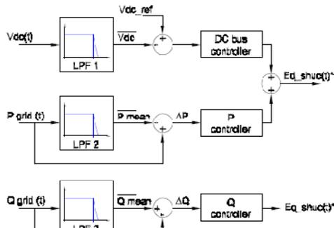
Fig.5.6 Shunt compensator controller
