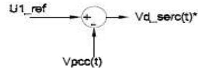
Fig.5.5 Series compensator controller
