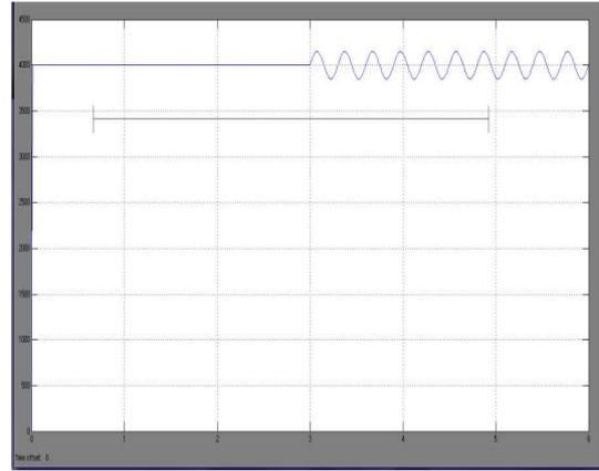
**Fig.6.7** Voltage of the capacitor in the DC-Bus
