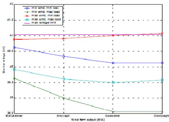
Fig.3.1 Example of voltage for feeder with and without wind power
