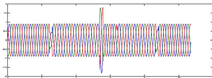
Fig.-7(c) Load Side Voltage after clearing the Voltage Sag and Swell
