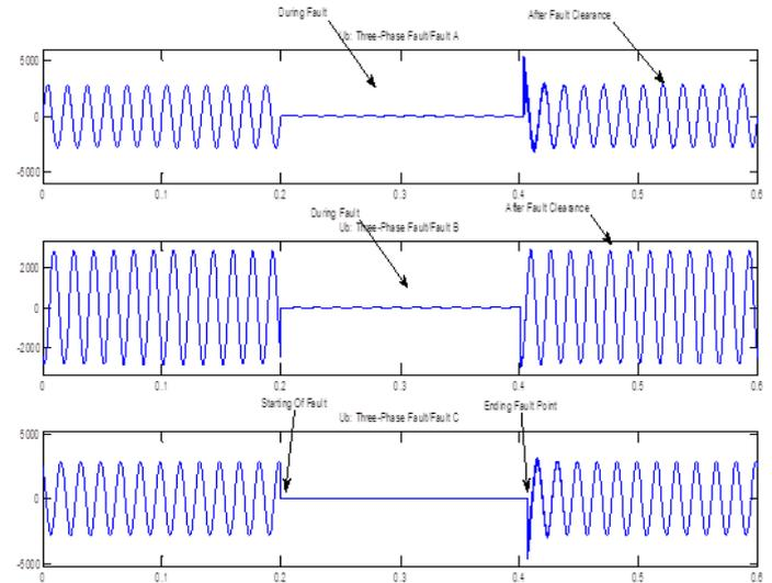
Fig.-8(a) Three phase fault without DVR
