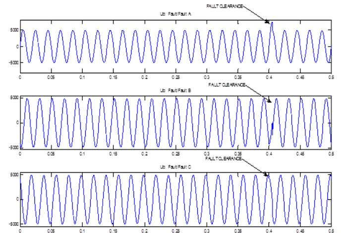
Fig.-8 Three phase fault with DVR voltage compensation
