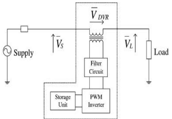
Figure-1: DVR series connected topology
