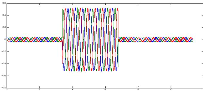
Fig.-6(b) Compensated Voltage injected by DVR
