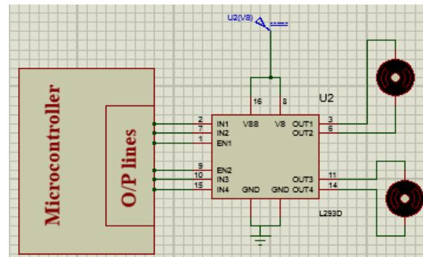
Fig. 5 Interfacing of DC motors
