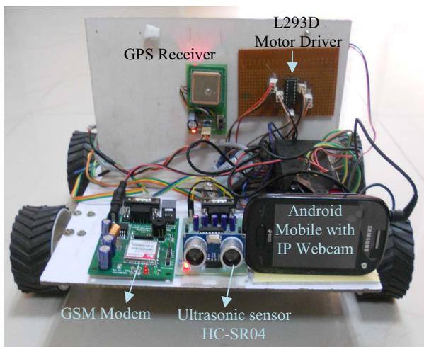
Fig. 11 Experimental Setup of Mobile Robot System (Back view)
