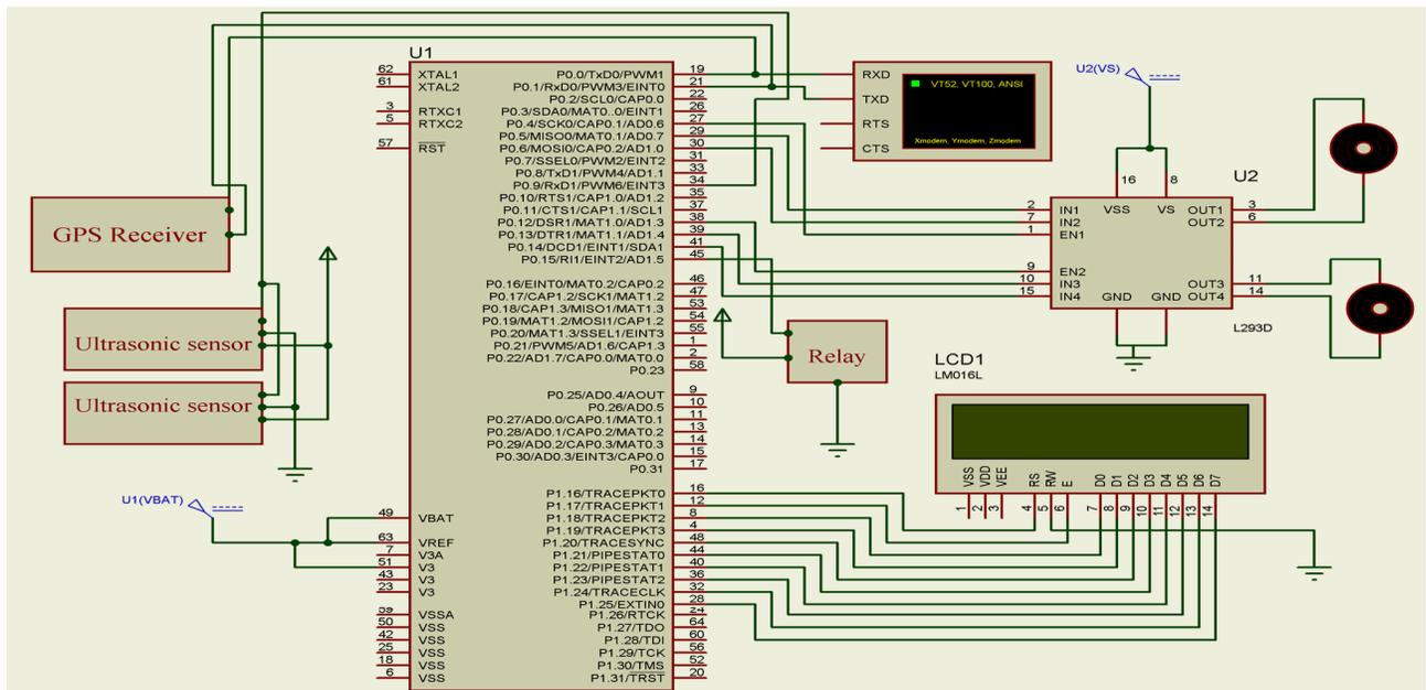
Fig. 9 Complete Schematic Diagram of the Proposed Mobile Robot System
