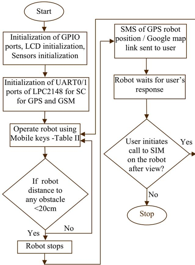
Fig. 7 Flowchart showing various events that occur at remote station
