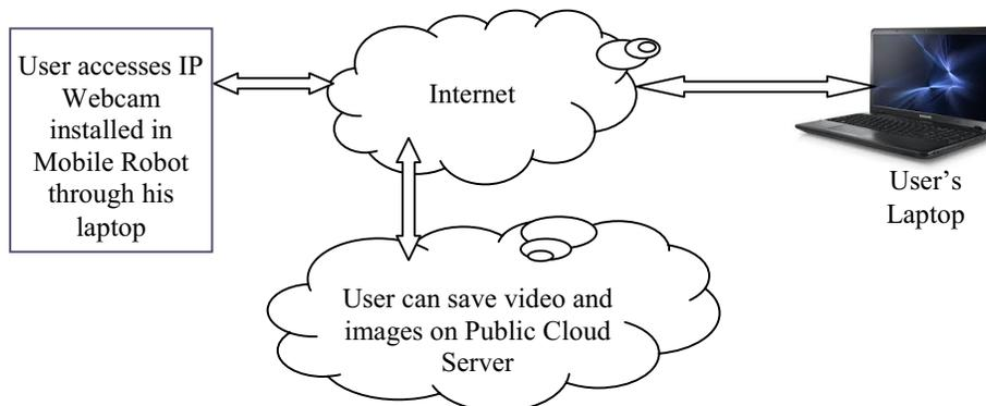
Fig. 2 Block diagram of Base station (User's side)
