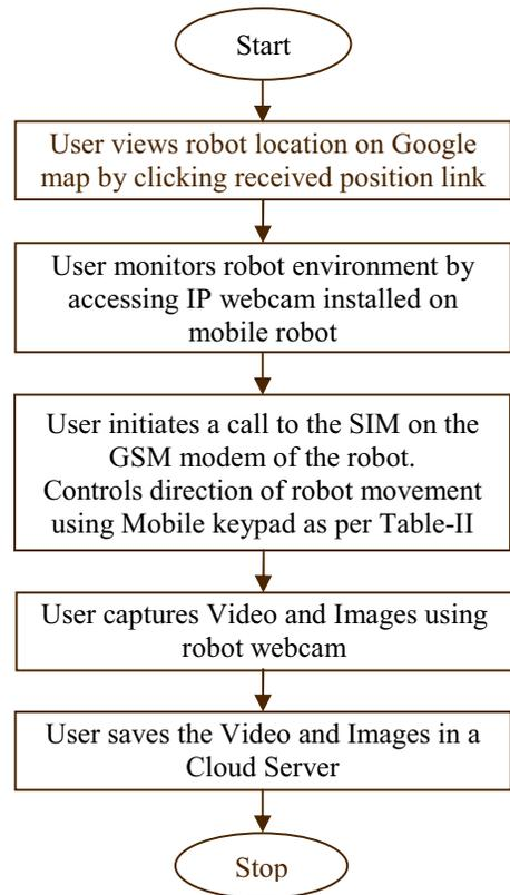
Fig. 8 Flowchart for Base station (User's side)
