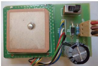
Fig. 3 Single Frequency GPS Receiver module
