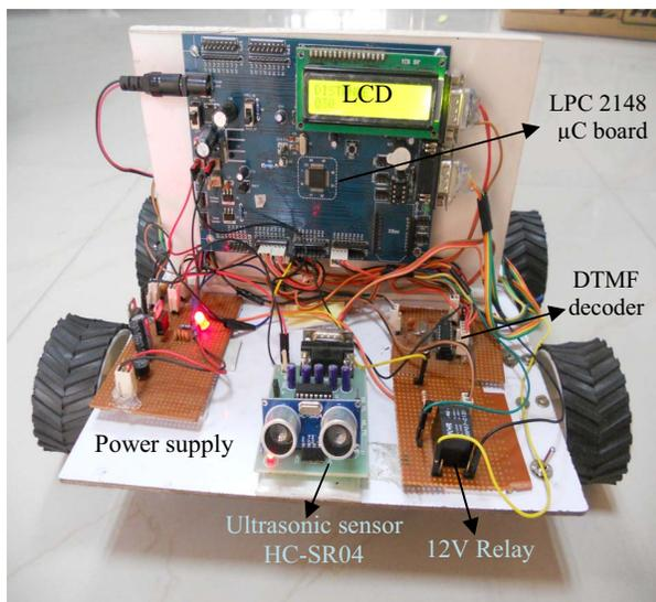
Fig. 10 Experimental Setup of Mobile Robot System (Front view)
