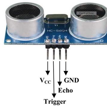
Fig. 4 HC-SR04 Ultrasonic Sensor
