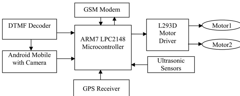
Fig. 1 Block diagram of Remote station (Mobile Robot)
