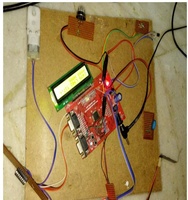
Fig.7 Prototype of the Transmitter section
