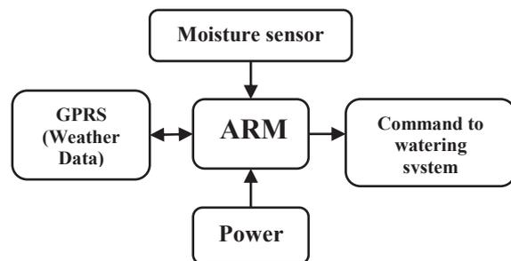
Figure 2. Block diagram of watering system
