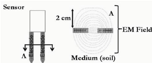
Figure 3. Capacitive active soil sensor
