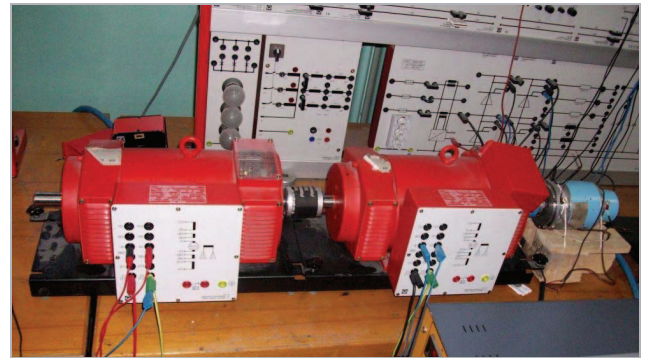
Figure 5. 1 kW LM brand DC motor and taco generator
