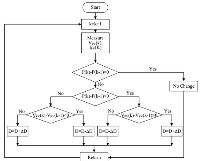
Fig. 3 Diagram of the P & O method.
