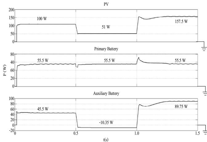
Fig. 12 Output power of the PV panel, the primary battery and the auxiliary battery in changed light intensity condition ( $500 \text{ W/m}^2$  -  $250 \text{ W/m}^2$  -  $700 \text{ W/m}^2$ ).
