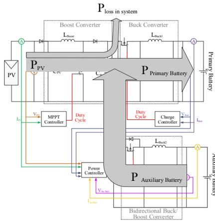
Fig. 7 Direction of the power transmission mode III.
