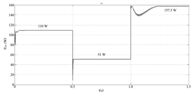
Fig. 10 The power of the PV panel in changed light intensity condition (500 W/m<sup>2</sup> - 250 W/m<sup>2</sup> - 700 W/m<sup>2</sup>).
