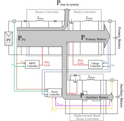
Fig. 5 Direction of the power transmission mode I.
