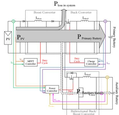
Fig. 6 Direction of the power transmission mode II.
