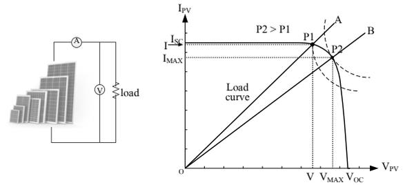
Fig. 2. The operation of the MPPT.
