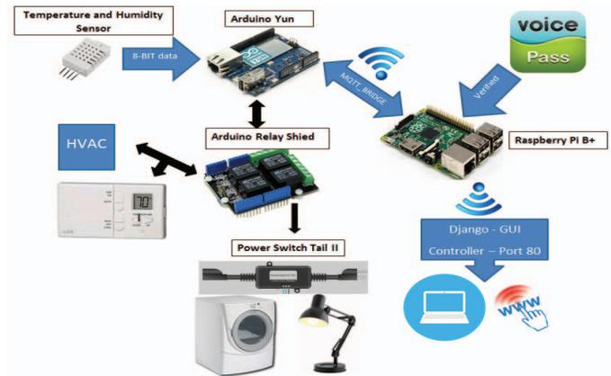
Fig. 1. Schematic of the Home Automation System.
