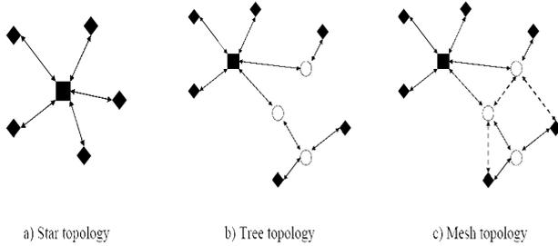
Figure 3. Different topologies of ZigBee network
