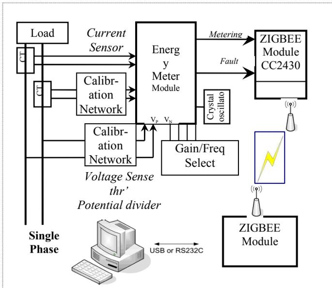
Figure 1. General Block Diagram Of The Scheme
