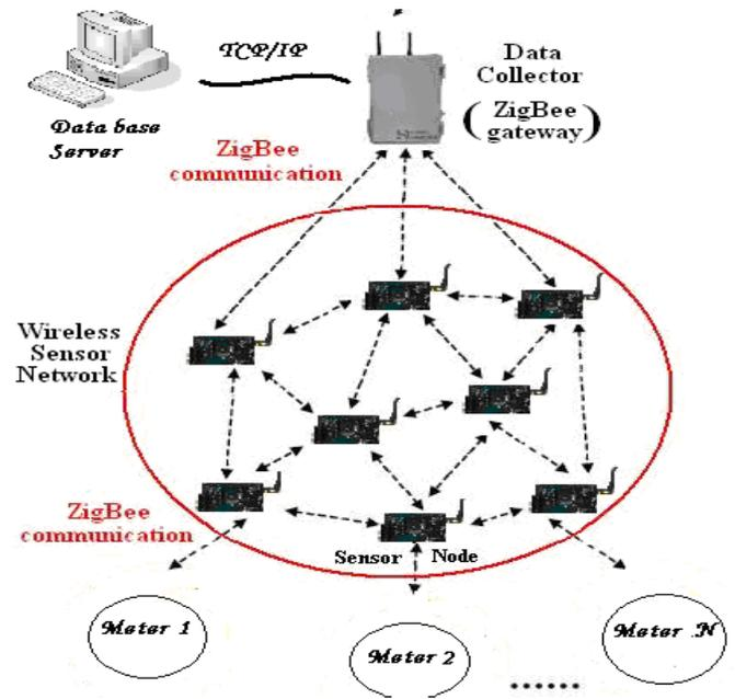
Figure 4. Long distance EM reading through ZigBee network
