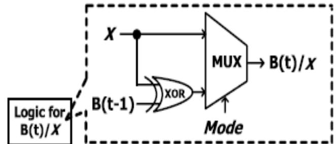
Fig.3.4 Balance logic-operation sharing of  $B(t)$  and  $X$
