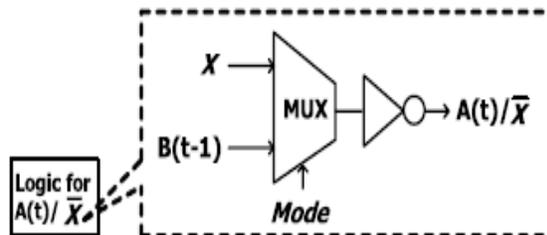
Fig.3.3 Balance logic-operation sharing of  $A(t)$  and  $X$
