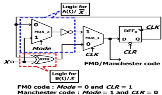
Fig.3.5 Unbalance computation time between  $A(t)/X$  and  $B(t)/X$
