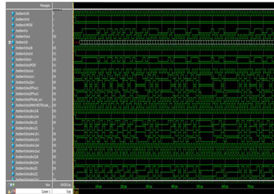
Fig 4.1 Implementation of Manchester Code Output Waveform
