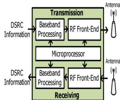
Fig. 2.1. System architecture of DSRC transceiver.
