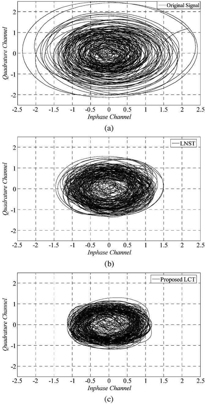
Fig. 3. (a) The original OFDM; (b) companded OFDM signal by LNST; (c) companded OFDM signal by the proposed transform.
