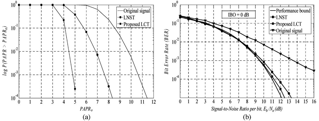
Fig. 6. Performance of LNST and proposed LCT. (a) Simulated CCDFs of LNST and proposed transform. (b) BER performance in nonlinear AWGN channel.
