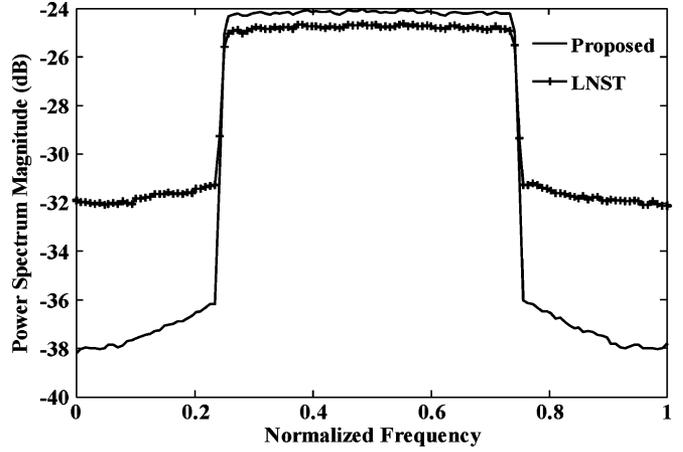
Fig. 4. Power spectrums of LNST and proposed transforms.
