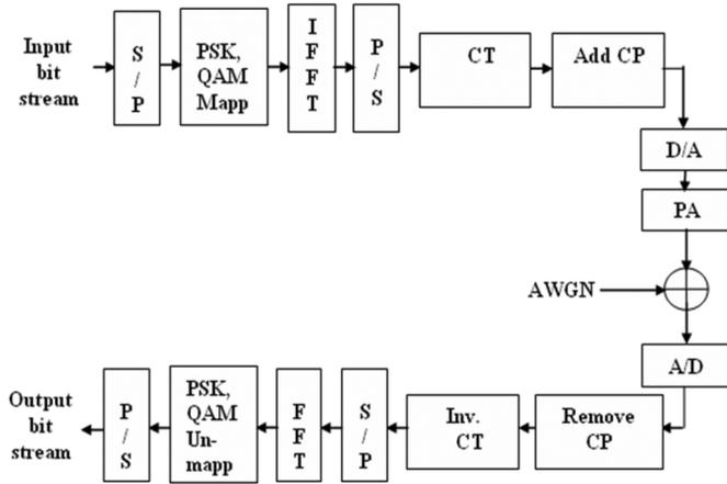
Fig. 1. Typical companded OFDM system.
