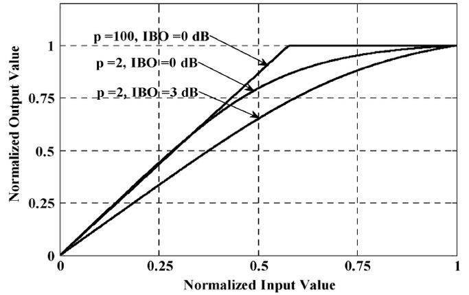
Fig. 5. SSPA characteristics.
