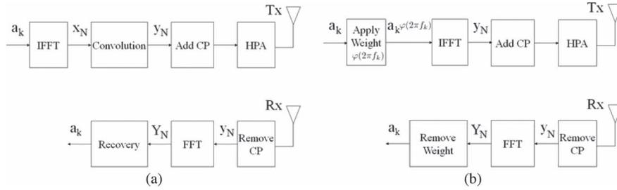
Fig. 1. Simplified block diagrams for an OFDM system with (a) convolution scheme and (b) proposed weighting scheme.
