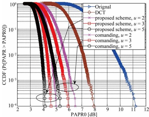
Figure 4. Comparisons of the CCDF of different PAPR reduction schemes.
