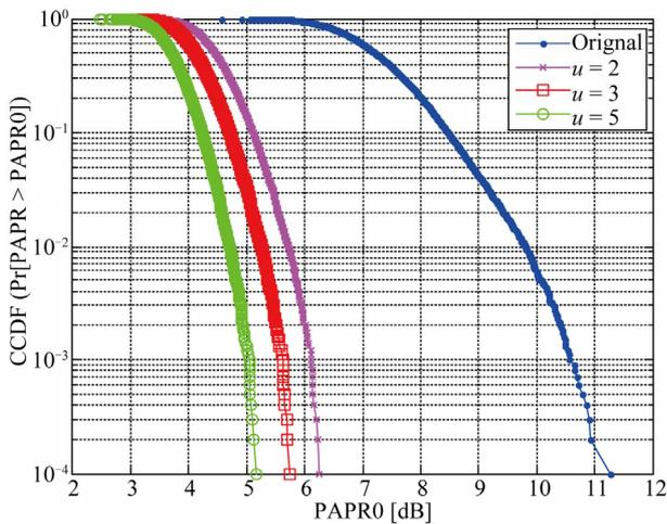
Figure 2. Comparisons of the CCDF of different companding factor  $u$ .
