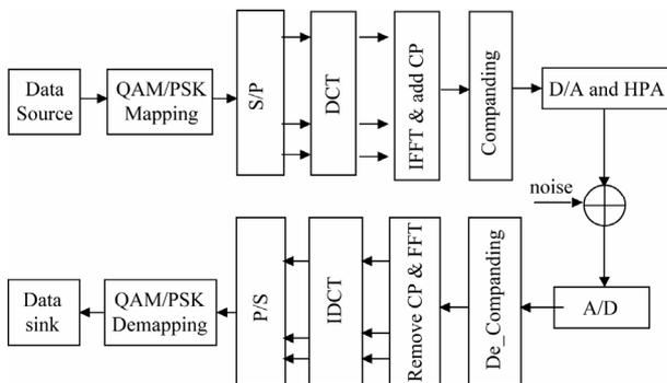
**Figure 1. OFDM system block with DCT-companding.**
