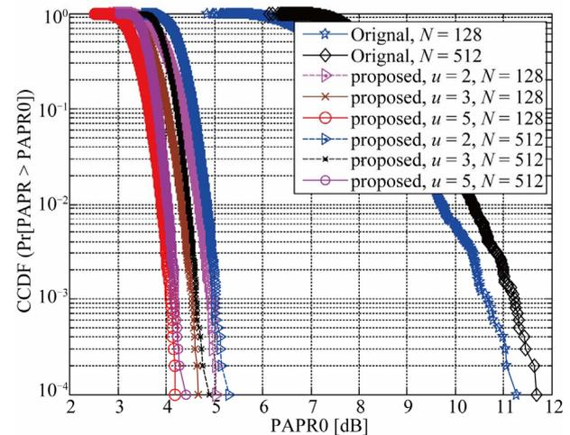
Figure 5. Comparisons of the CCDF of proposed scheme with different subcarriers.
