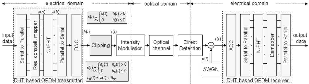
Fig. 1. DHT-based O-OFDM: schematic including Gaussian noise. Clipping is illustrated for AC signals and DC-biased signals with residual negative peaks.
