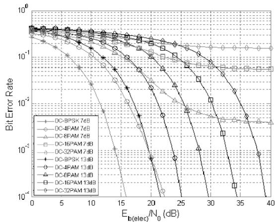
Fig. 3. BER versus  $E_{b(elec)}/N_0$  for DHT-based DCO-OFDM with 7 and 13dB bias.
