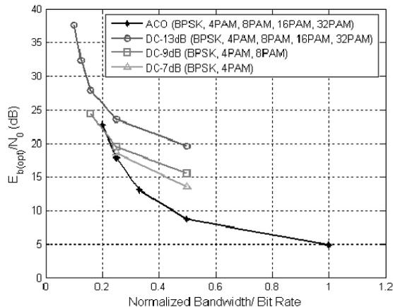
Fig. 4.  $E_{b(opt)}/N_0$  versus normalized bandwidth at  $10^{-3}$  BER for DHT-based AC and DC-biased (with 7, 9 and 13dB) O-OFDM. Each point indicates a constellation size (the smaller the size, the larger the normalized bandwidth).
