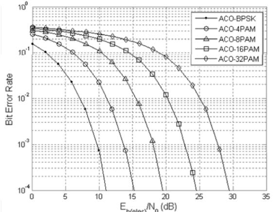
Fig. 2. BER versus normalized bit electrical energy for DHT-based ACO-OFDM using different real constellations (BPSK, 4, 8, 16, 32 PAM).
