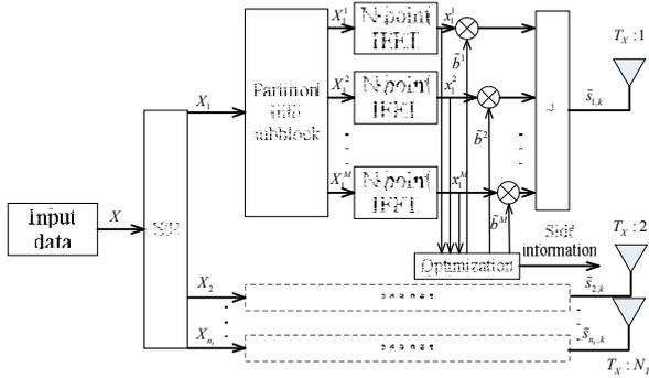
Fig.1 The block diagram of PTS scheme in MIMO-OFDM
