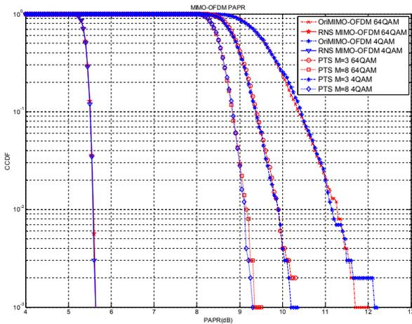
Fig.3 PAPR reduction performance of the proposed scheme, PTS scheme and the conventional MIMO-OFDM with  $N=2048$ , 4QAM/64QAM  $V=3$ ,  $W=\{-1, 1\}$ ,  $M=3/M=8$ .
