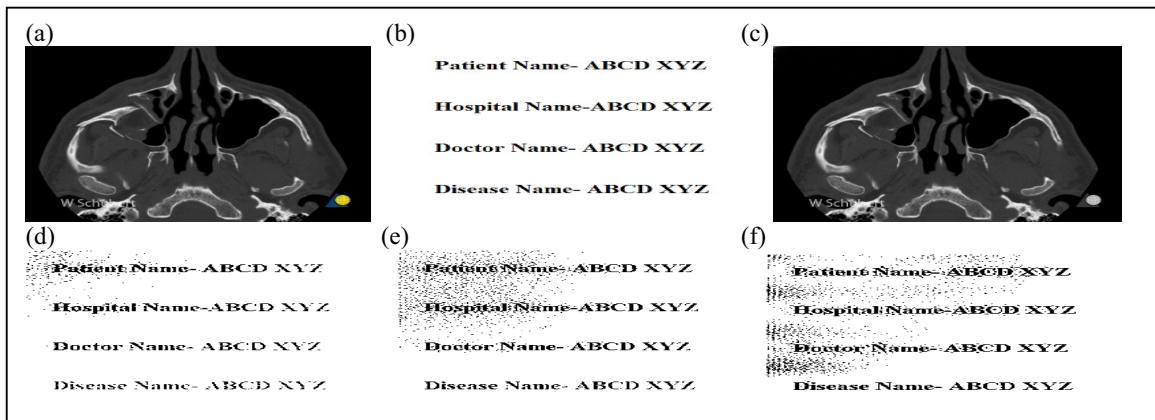
Fig. 3: CT scan watermarked result images (a) Original Image; (b) Watermark Image; (c) Watermarked Image; (d) Recovered Image for 0.5\alpha ; (e) Recovered Image for \alpha and (f) Recovered Image for 2\alpha .
